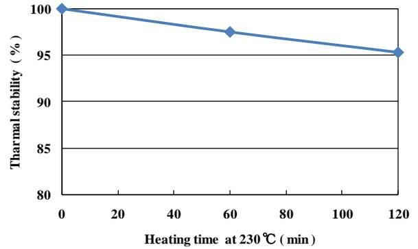
Figure 5. Thermal stability of the retarder at 230 °C.
