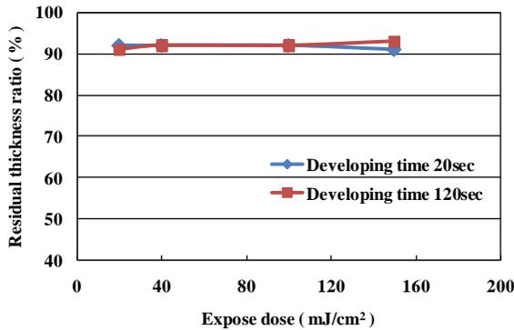
Figure 3. Dependence of residual thickness ratio on Expose dose in change of developing time.
