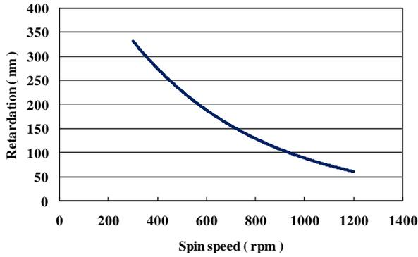
Figure 2. Dependence of spin speed on retardation of the retarder.
