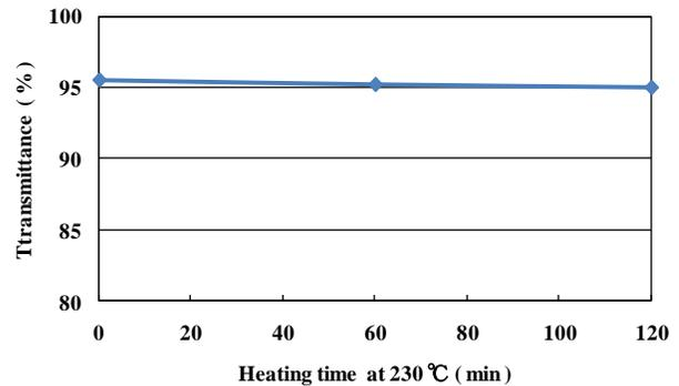
Figure 6. Transmittance (400 nm) of the retarder at 230°C.
