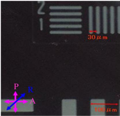
**Figure 7. Polarizing microscopic photograph of the Patterned retarder prepared by Alkali development under crossed polarizers.**
