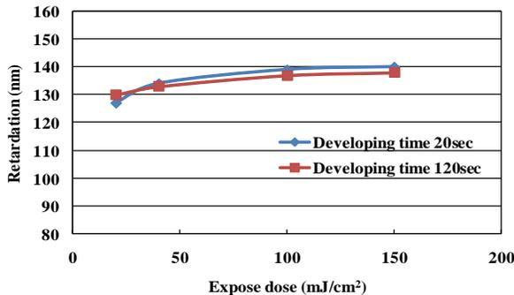
Figure 4. Dependence of retardation on expose dose in change of developing time.
