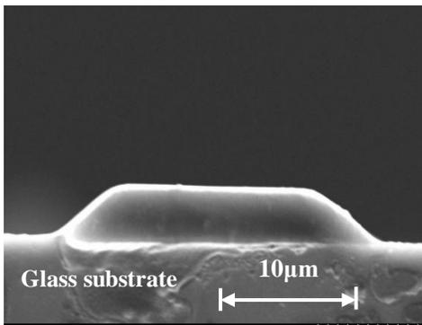
**Figure 8. SEM image of cross sectional shape of patterned retarder.**
